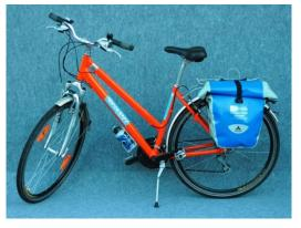
Aluminium frame, Shimano gear system with "rapid-fire" shifters, 21 speed, Rack on back with 1 rear pannier, Repair kit, Lock, Cycling odometer
