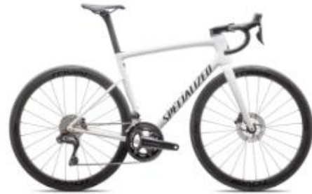
ROAD 3 Specialized Tarmac SL8 EXPERT 2025 New! Description: Full carbon frame / Carbon rims. Gear: Shimano Ultegra Di2 (2x12) 52/36T · 11/30T Sizes: 44 / 49 / 52 / 54 / 56 / 58
