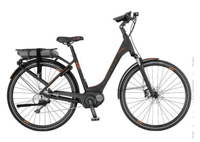
Frame types unisex and low step Sizes 17,19 in / 44,48 cm Front suspension Stand Mud guards Luggage rack Bottle holder Computer meter Front gear set 3 (48,38,28) Back gear set 7 (28,14) E-gears Brakes V-brake Motor in mid section Battery authonomy80 km at 50% use
