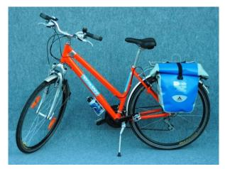
Aluminium frame Shimano gear system with "rapid-fire" shifters: 21 speed Lock, Rack on back, 1 rear pannier, Repair kit
