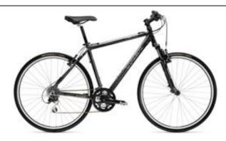
We use Trek FX3 Hybrid 27 speed touring bike with aluminium frame and Shimano gear system.
